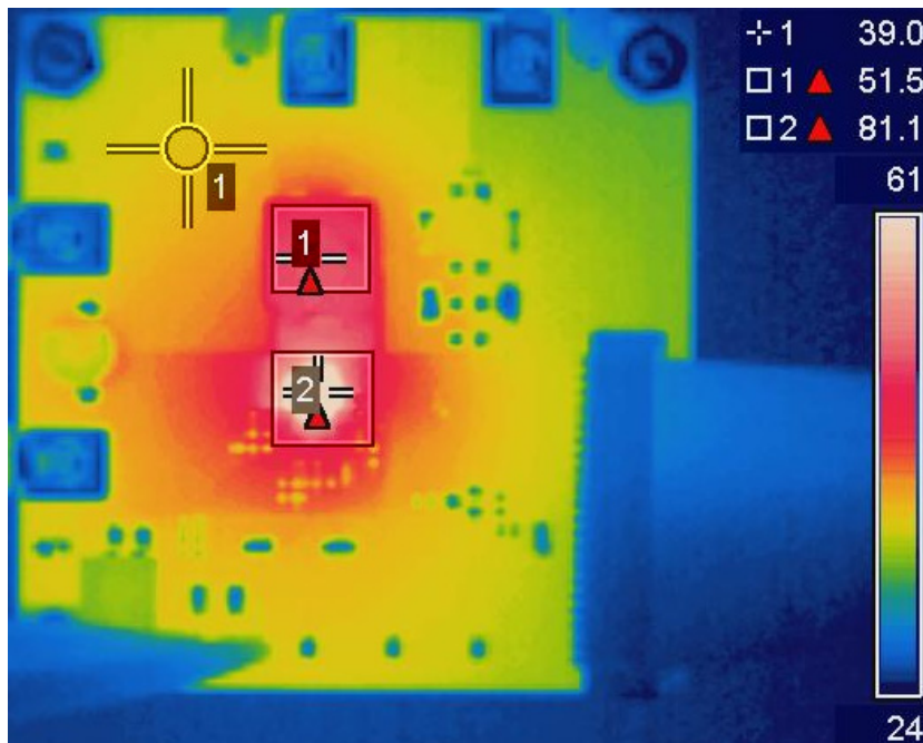
Fig. 17: Thermal Image (IR3865: 81°C, Inductor: 52°C, PCB: 39°C)
